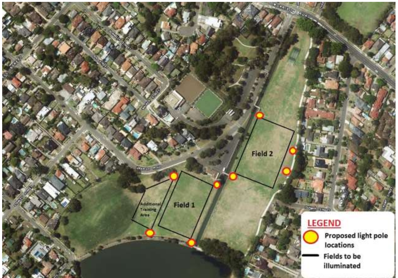
Figure 1 – Proposed location of the light poles at Morrison Bay Park sports field.
