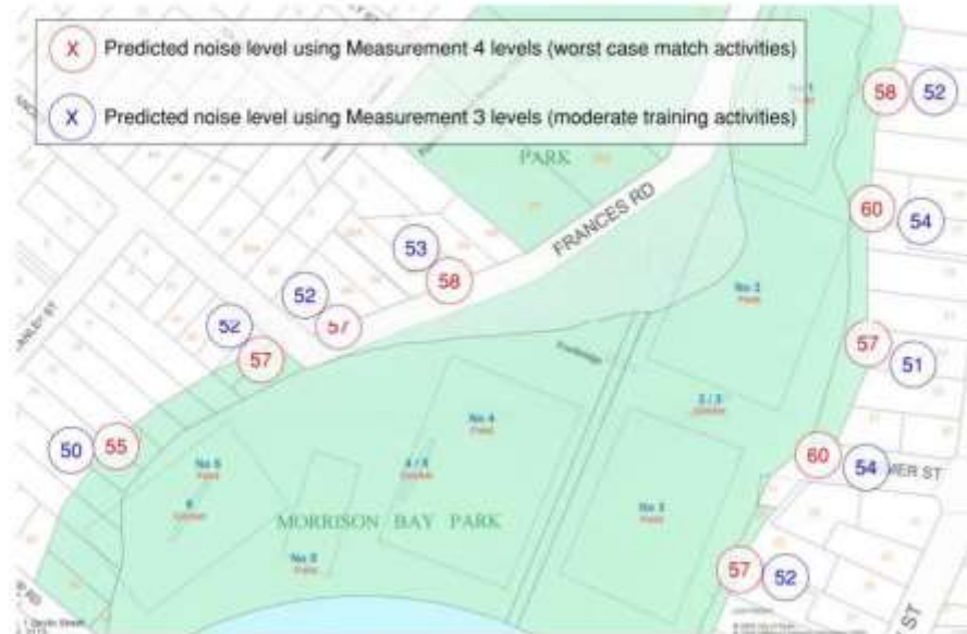
Figure 5: Predicted noise levels for worst case and moderate training activities at Morrison Bay Park for Original Lighting Proposal
