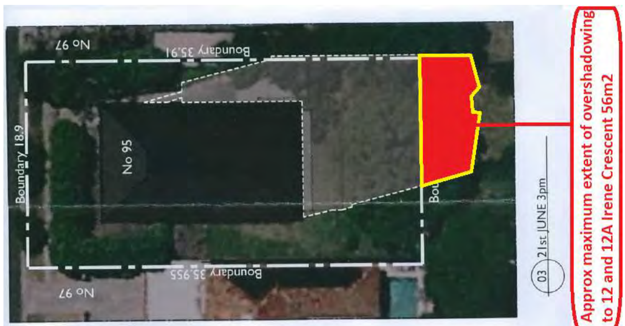
Figure 5 Submitted shadow diagram at 3pm illustrates extent of shadows (shaded in red) to properties to the rear, approximately 56m 2 . Source: Submitted shadow diagram edited for use by CPS
