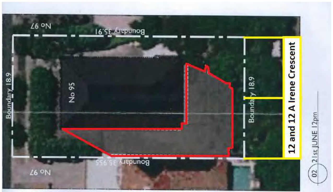
Figure 4 Submitted shadow diagram at 12pm illustrates no shadows (outlined in red) to properties to the rear (indicative boundaries in yellow) Source: Submitted shadow diagram edited for use by CPS
