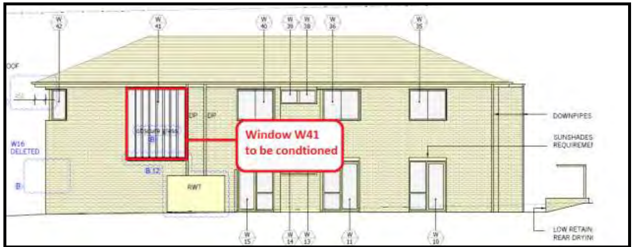
Figure 12 Side facing stairwell window on western elevation to be conditioned to incorporate obscure glazing
