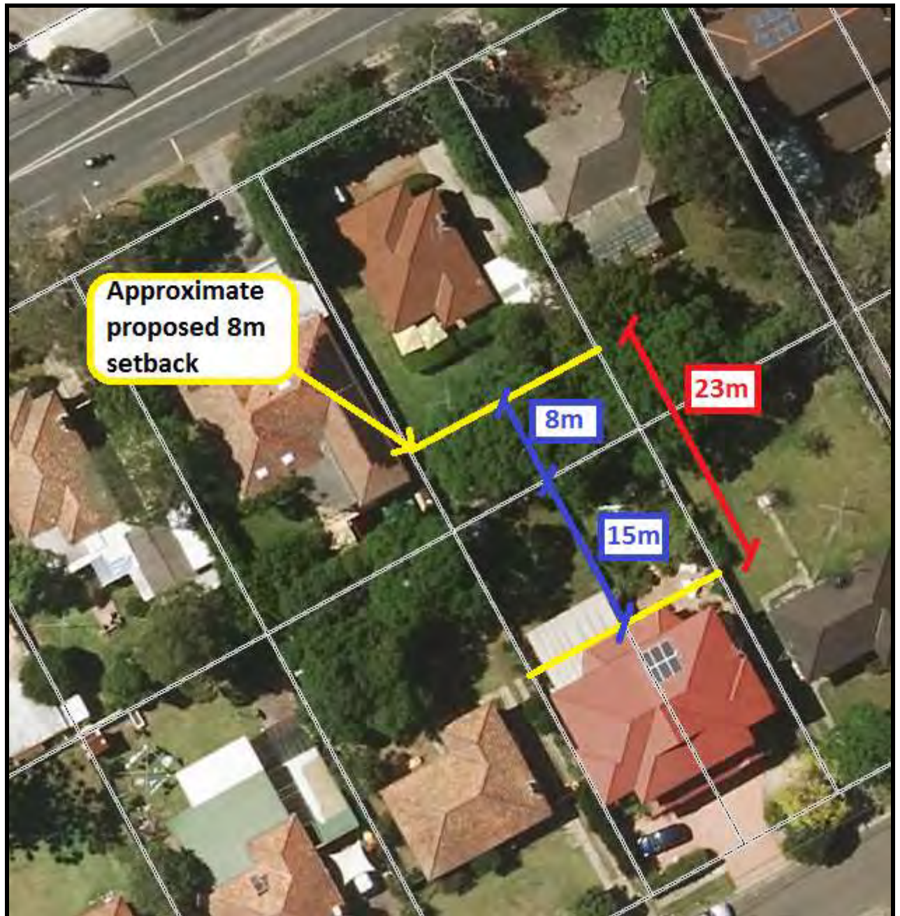
Figure 2 - Proposed 8m setback in relation to existing 15m setback of 12 and 12A Irene Crescent. Total building separation of 23m.
