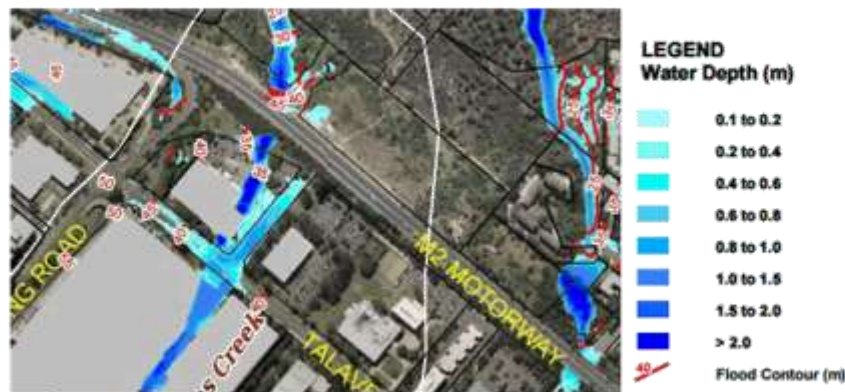
Figure 19 1 in 100 year flood event Source: City of Ryde – Macquarie Park Floodplain Risk Management Study and Plan
