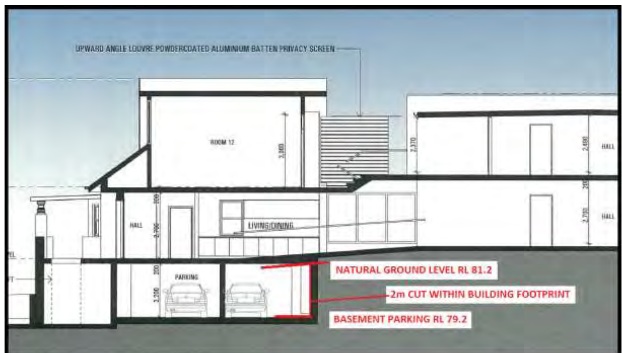
Extract of Section AA – Showing cut within the building footprint of max 2m (at location of basement).
