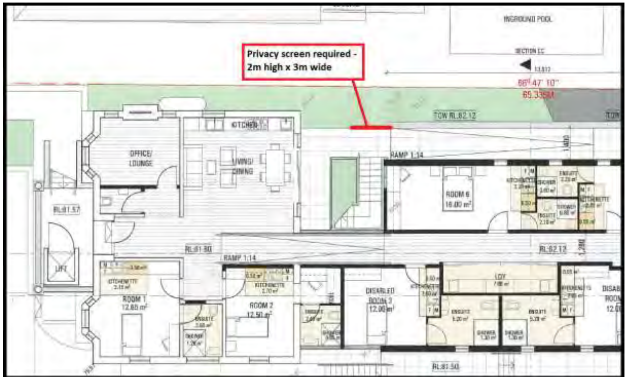
Plan showing location of privacy screen to prevent overlooking as occupants travel down the lower section of the stairs
