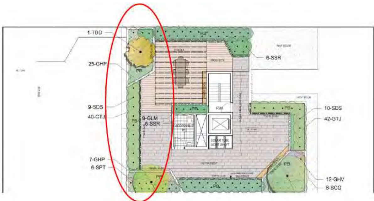
Figure 6: Rooftop terrace showing landscape screening along western elevation
