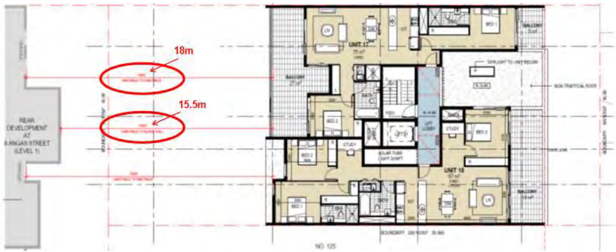
Figure 5: Level 6 floor plan showing distance separation to building A at 4 to 8 Angas Street
