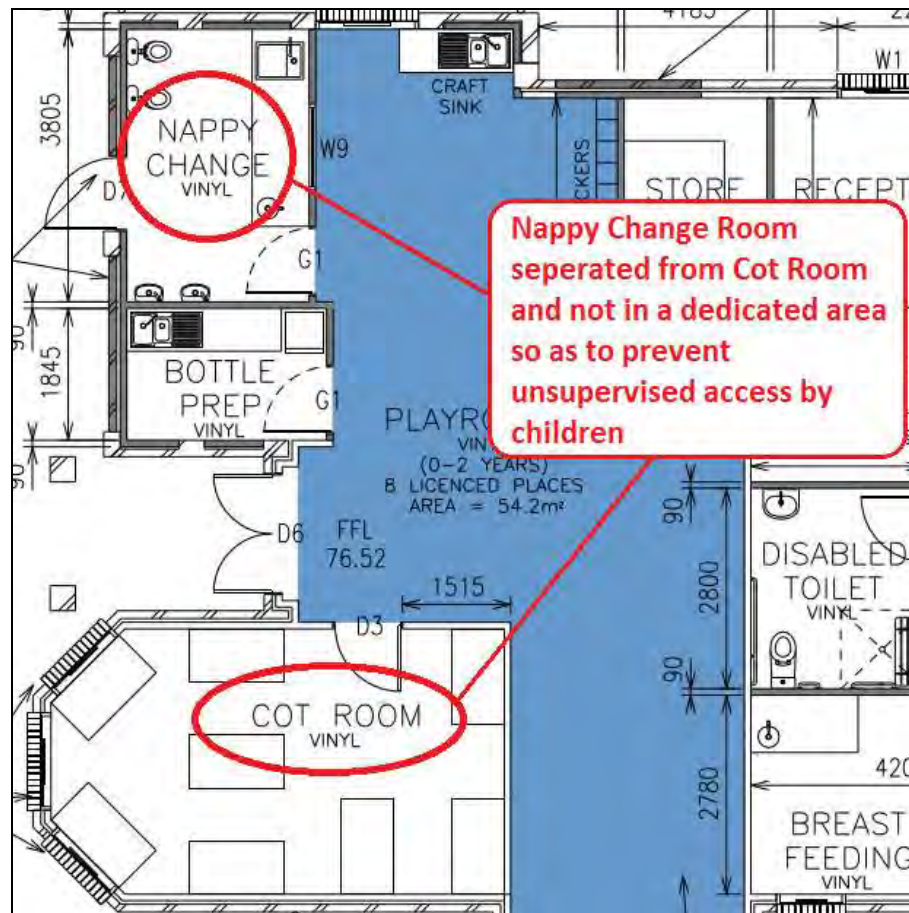
Extract of ground floor plans demonstrating the Cot Room and Nappy Change Room not being located adjacent to each other and also possible unsupervised access to the Nappy Change Room. Source: Ground Floor Plan by applicant, edited for diagrammatic purposes by CPS
