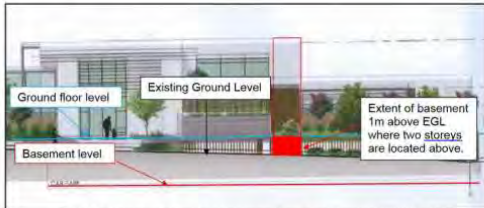
Figure 4 – Diagram indicating the approximate extent of the basement above the existing ground level at the Macpherson Street elevation
