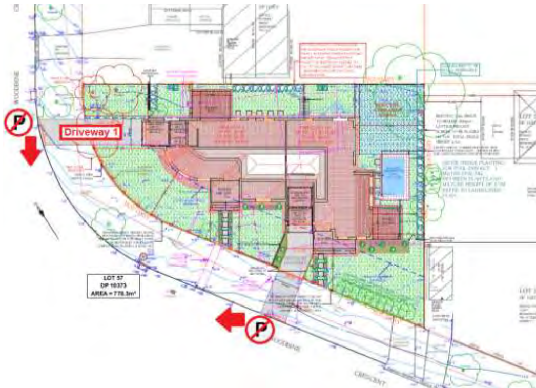
Figure 4 – Site plan of proposed development showing location of Dwelling 1 driveway & no parking zone.
