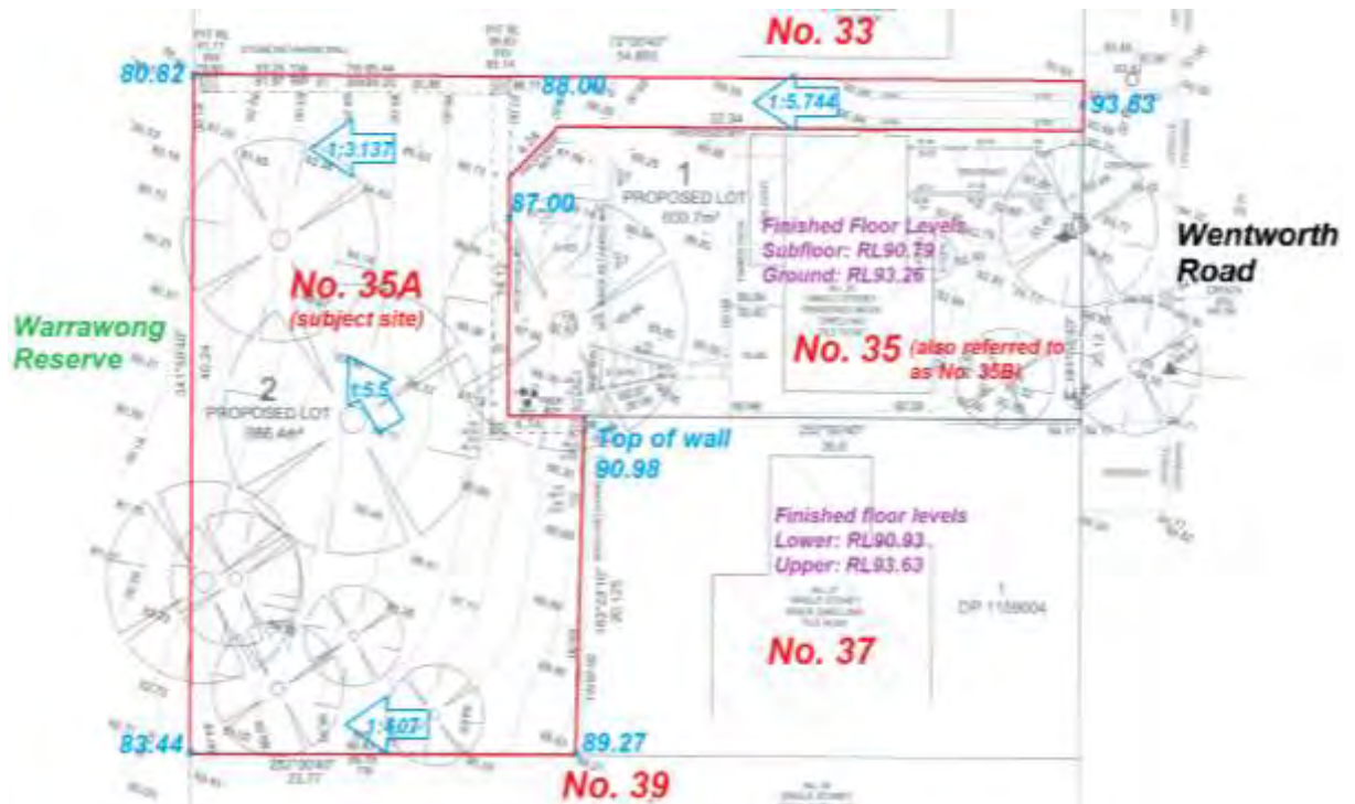
Figure 3. Site survey showing gradients and site levels across the site (Source of finished floor levels of neighbouring dwellings from LDA 2014/560 and LDA 2012/26 applying to the dwellings at No. 35 and 37 Wentworth Road respectively)
