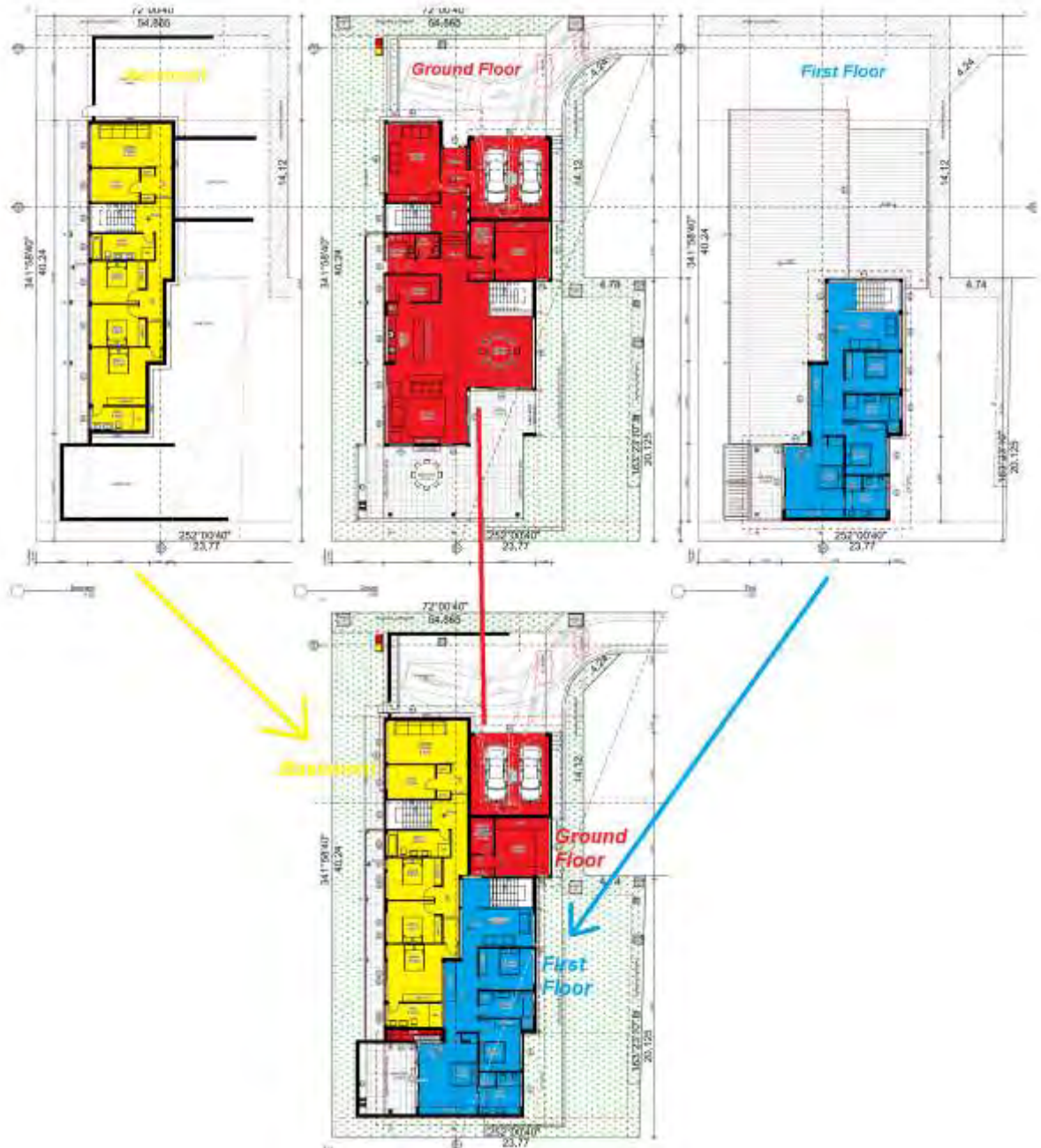
Figure 6. Floor plans overlaid on the ground floor plan to show number of storeys
