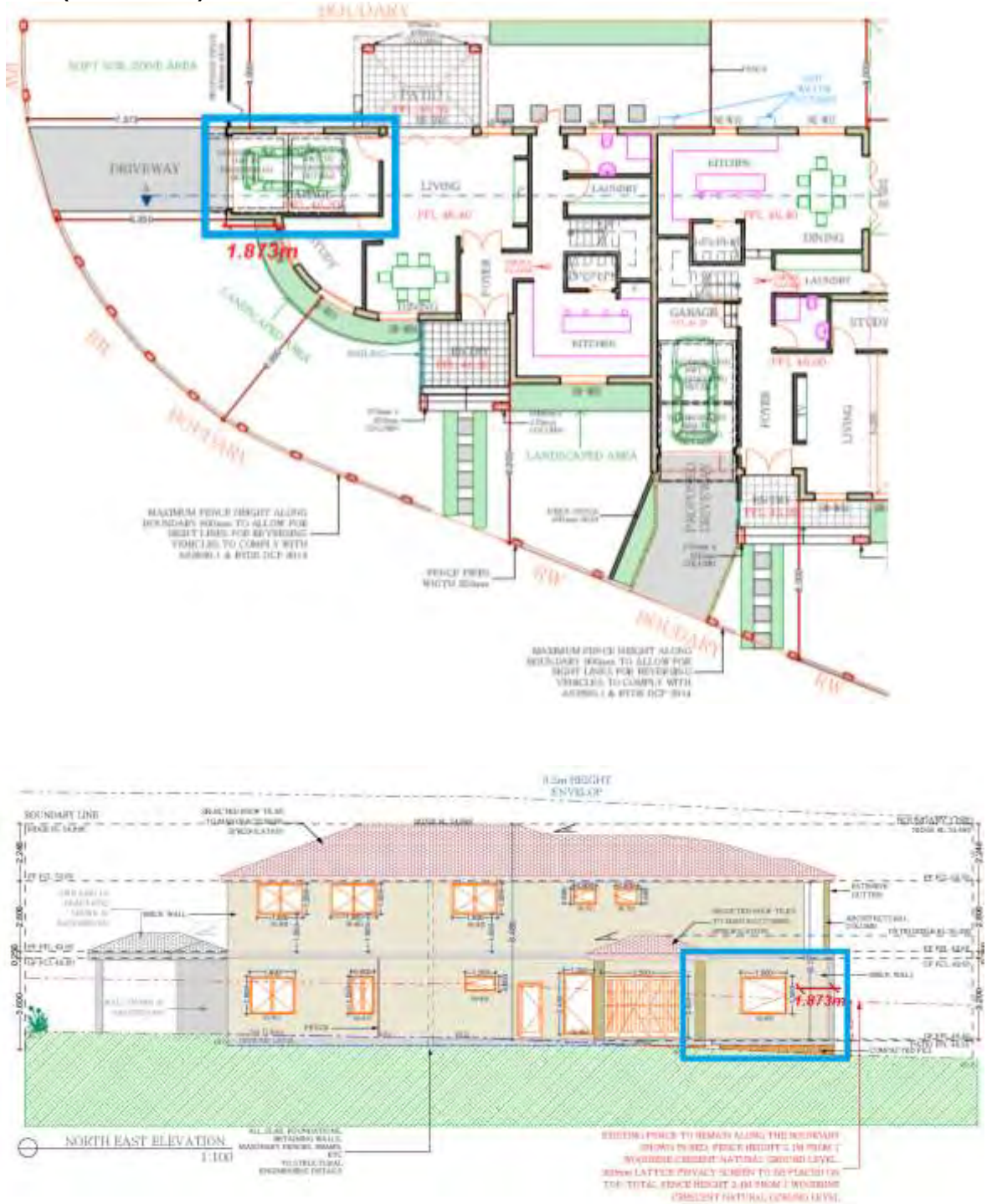
Figure 12 – North east elevation plan and ground floor of the proposed development showing area where garage sits in front of the dwelling facade Source: Applicant submitted plans—edited by Assessment Officer
