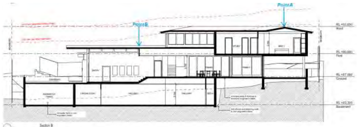
Figure 4b. Long section of proposed dwelling (Source: Submitted Plans – Revision D)
