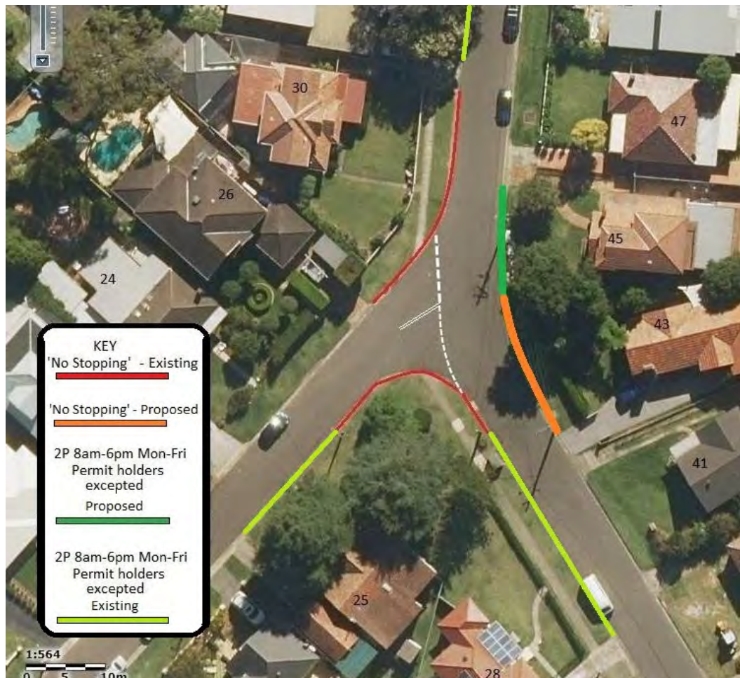
Figure C2 Proposed intersection treatment
