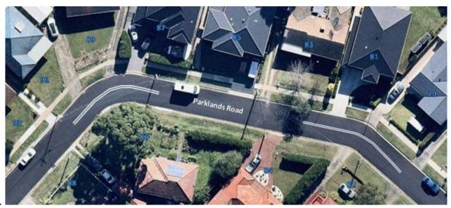
Figure 2: Proposed Location of Double Barrier Lines
