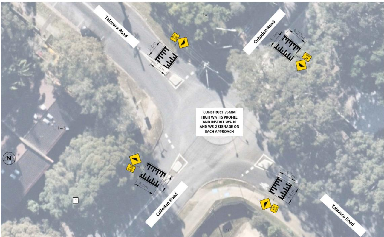
Figure 2 – Location of proposed speed humps at the intersection of Culloden Road and Talavera Road
