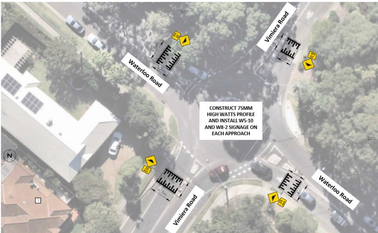
Figure 4 – Location of proposed speed humps at the intersection of Vimiera Road and Waterloo Road
