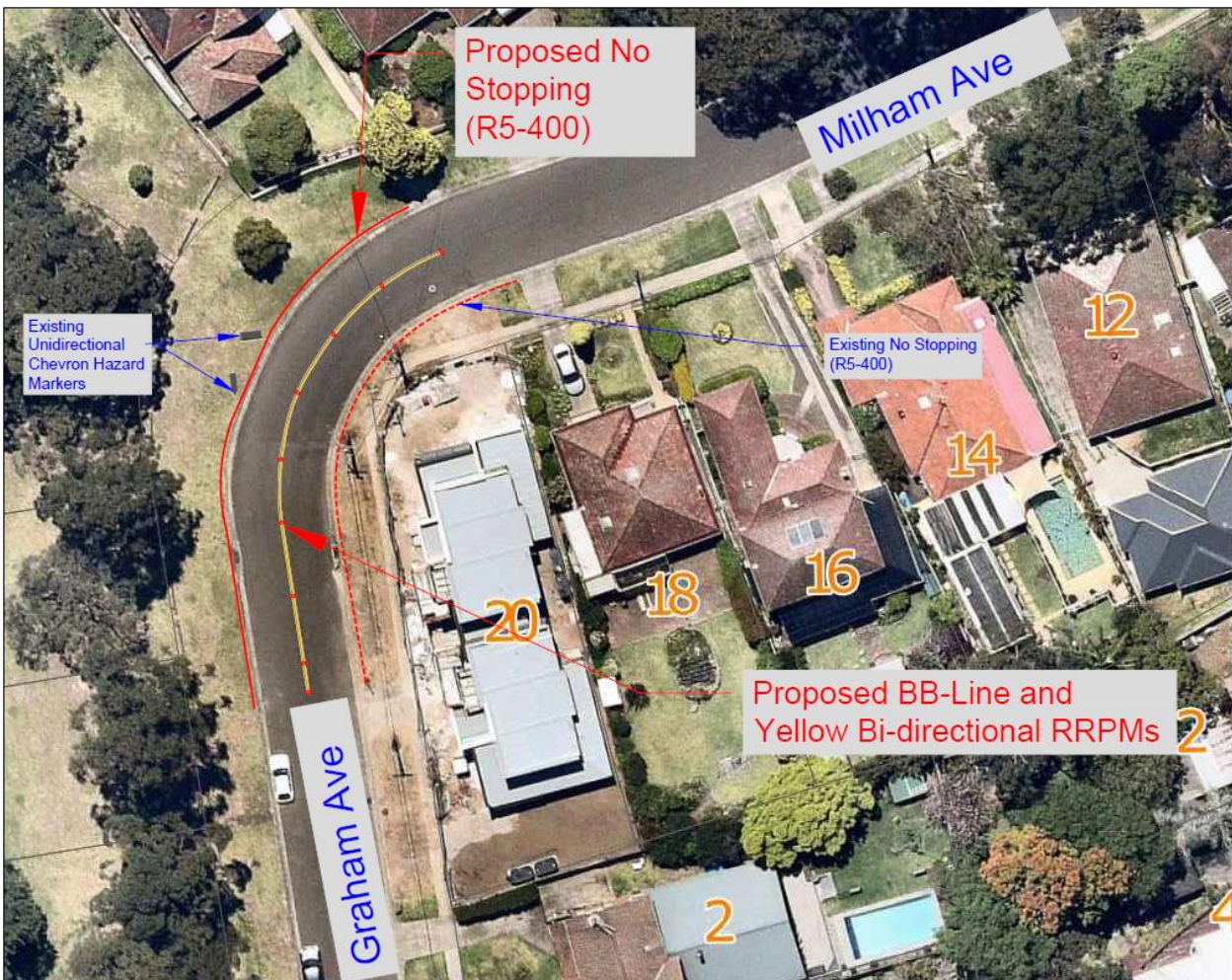
Figure A2: Proposed upgrade to signage and delineation through the 90 degree bend
