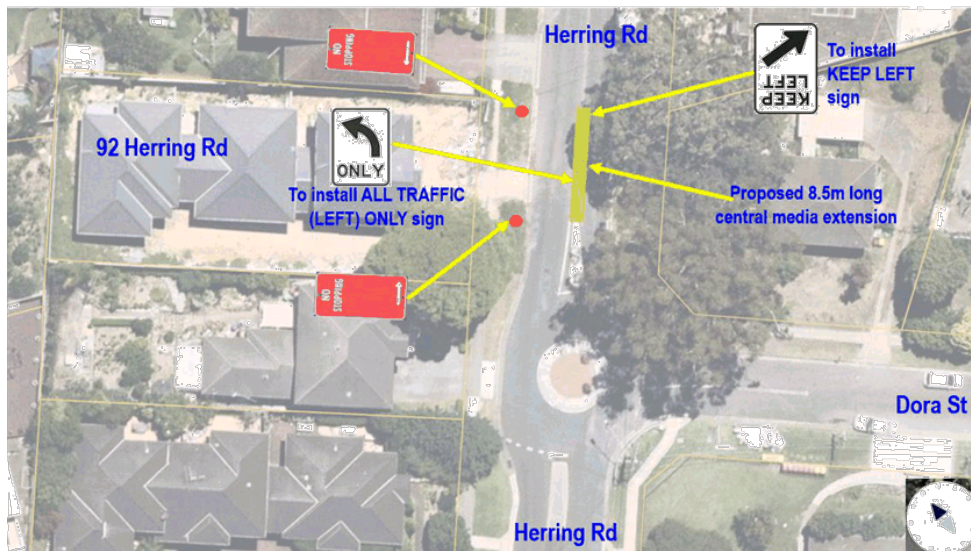
Figure 2: Proposed raised median island along the property frontage on 92 Herring Road, Marsfield.
