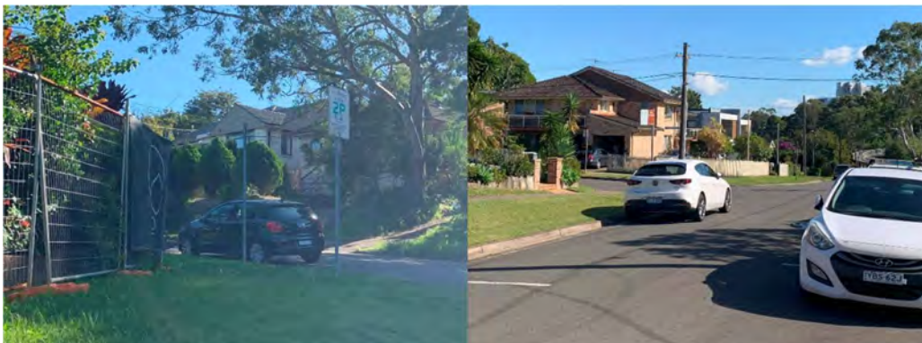
Figure 5-4: Visibility obstruction from parked cars at the Trevitt Road / Lane Cove Road and Paul Street / McGregor Street intersections
