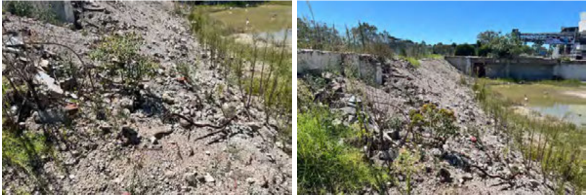
Figure 3 - photos showing the presence of steel, bricks, plastics etc in soils.
