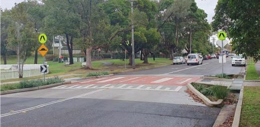
Figure 4 – Example of a raised pedestrian crossing on Ryde Road in Gladesville
