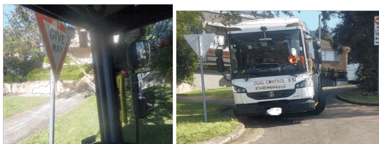
Figure 14: The truck is only just able to clear the GIVE WAY sign at the end of the loop road. The driver advised that this was previously impacted.
