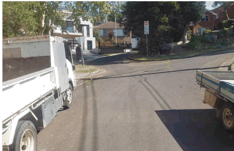
Figure 2: Looking towards the commencement of the loop road at chainage 0. With the truck parked on the left-hand side of the road, this severely limits the turning arc that is achievable to turn right into the one-way loop road – note the protruding wing mirror and risks of impacting it. Often bins are placed at point 2 and are inaccessible via a single forward movement. The truck driver must advance to point 1, and then reverse into place to access the bin at point 2. View from inside the truck.
