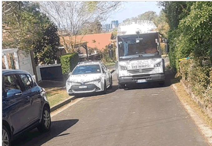
Figure 7: A view from outside the truck at chainage 130 showing (i) if the parked car did not straddle the kerb, there would not be sufficient passing clearance for all vehicles (let alone trucks); (ii) the lack of operating space for the bin pick up and set down.
