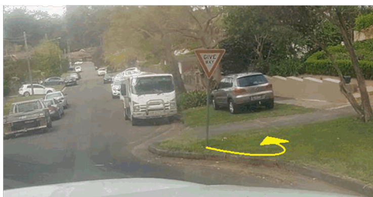
Figure 28: Chainage 368. The GIVE WAY sign should be shifted to the right as shown to reduce the risk of nuisance impacts.
