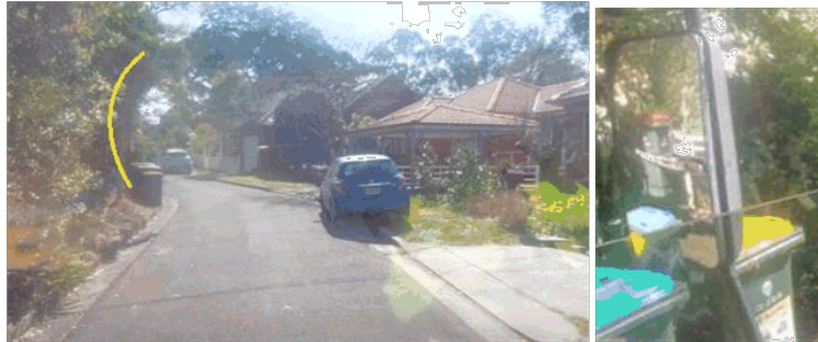
Figure 6: At chainage 105, when the truck cannot distance itself from the bins, usually as a result of parked cars such as that shown above, there is more demand for operating width behind the bin. As discussed previously, the lift-arm of the truck extends outwards initially before grabbing the bin. It then has a circular path as it is lifted above the truck. The yellow line is the indicative circular path of the bin as it is lifted and set down. Views from inside the truck.
