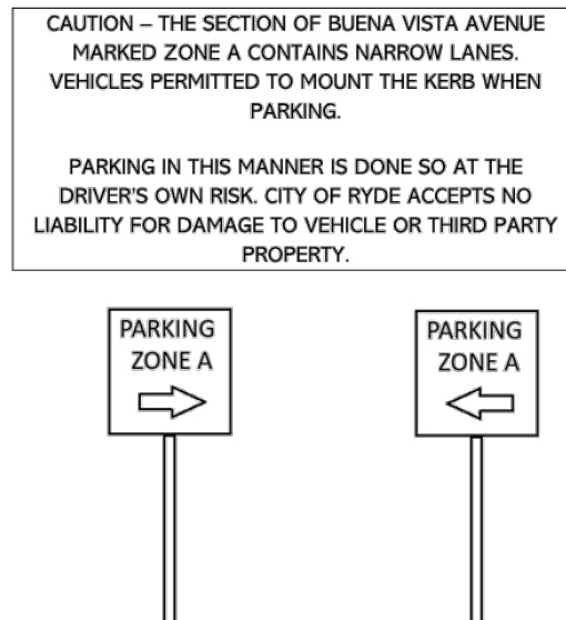
Figure 16: Top image - The CAUTION sign that could be installed at the start of, as well as at several points throughout Zone A. Bottom image – The boundary signs to Parking Zone A. Note that these should be placed on the residences side of the road and the arrow should point in the direction which Zone A lies in.
