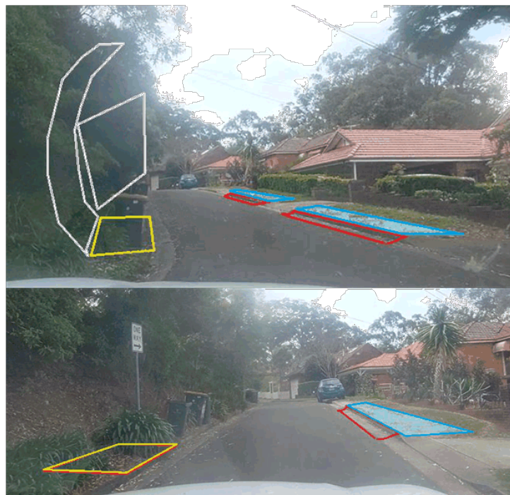
Figure 19: Chainage 60-105 showing the recommended rolltop kerbs in red, the hard stand areas for kerb-straddle parking in teal, and the tree pruning works in white. The bin hard stand is also shown in yellow. The curved shape of the vegetation clearing refers to the need to maintain a kinematic envelope for the lift arm of the truck and bin as it is lifted and set back down.
