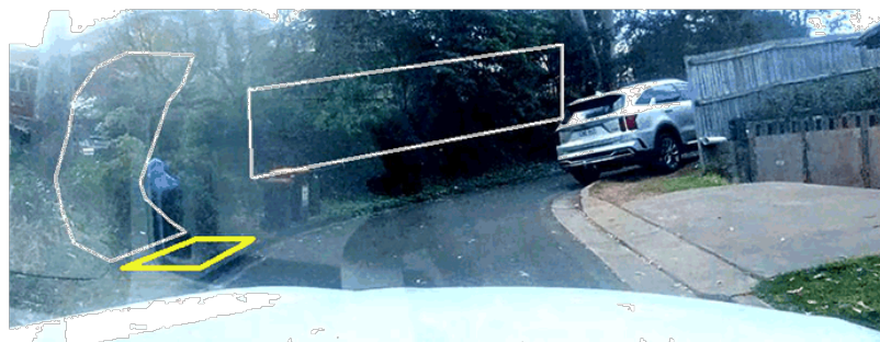
Figure 17: Chainage 0-20 of the loop road. A formalised bin hard stand area should be provided opposite the driveway to reduce the obstructions when accessing this bin. Tree pruning works should be carried out to improve the kinematic envelope of the waste collection truck.
