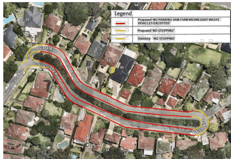
Figure 15: The parking restriction signage scheme as proposed by Council.
