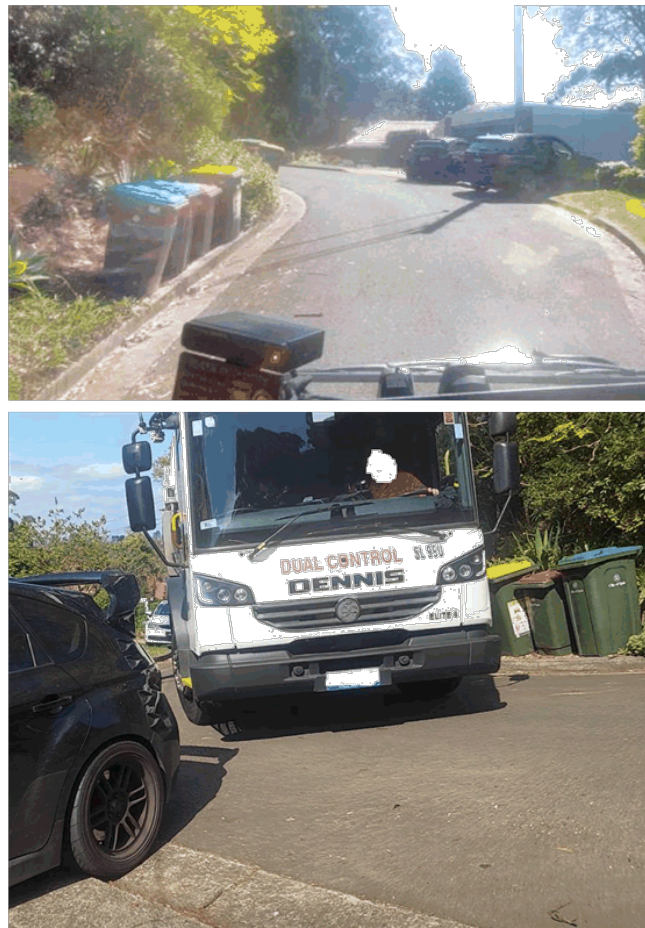
Figure 8: Photos taken from chainage 170. Top – A view from the truck cabin. Note the lean angle of the bins and the risk of these toppling. Note also the cars parked in the driveways which extend back into the trafficable area of the roadway and hence limit the manoeuvring space in approach to and throughout this curve. The driveways are very steep and have abrupt changes in grade such that “bottoming out” is a high risk. As such, car owners have resorted to this method of parking. Bottom - A view from outside the truck showing its lack of offset from the parked cars and the difficulty in accessing bins due to the angle of the truck body.
