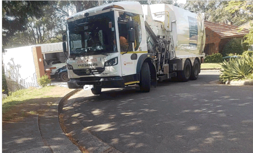
Figure 9: Note the width footprint of the truck as it negotiates the 180° hairpin curve. For an unimpeded run, the whole road width needs to be unoccupied at this point. Note also the angle of the truck relative to the inside kerb, which means the lift-arm is not always perpendicular to the kerblines. Most residents would assume that bins should be placed perpendicular to the kerblines. With parked vehicles in place, the driver most often needs to perform a three-point turn including one downhill reversing adjustment. As previously noted, if the truck mounts the inside kerblines, this most often lifts the rear left-tyres off the ground. These are the drive axles.
