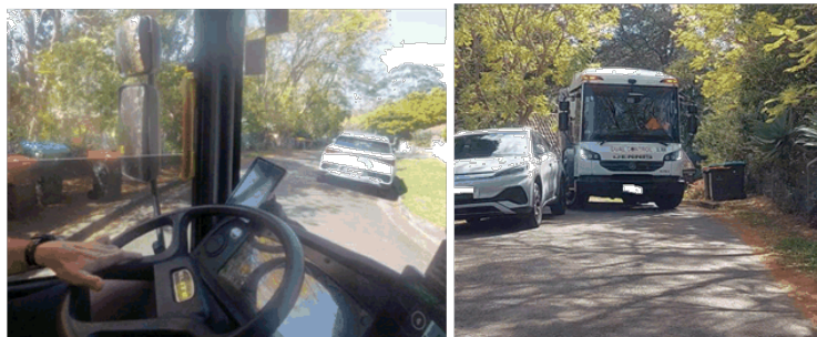
Figure 10: At chainage 195, the bins placed immediately downstream of and on the inside of the 180° curve, are difficult to access by the truck. The left-hand image shows the distance of the bins from the truck body due to its angle to the inside edge of road when turning. Note also the parked car as an additional obstruction. The right-hand image shows a view from outside the truck showing the lack of offset from the parked car. This shift-left movement was required immediately downstream of the 180° curve and immediately after collecting the bins.
