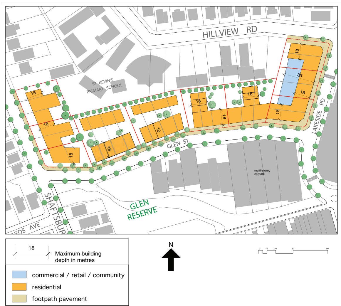
Figure 4.1.16 Glen Street and Lakeside Road Building Depth Control Drawing
