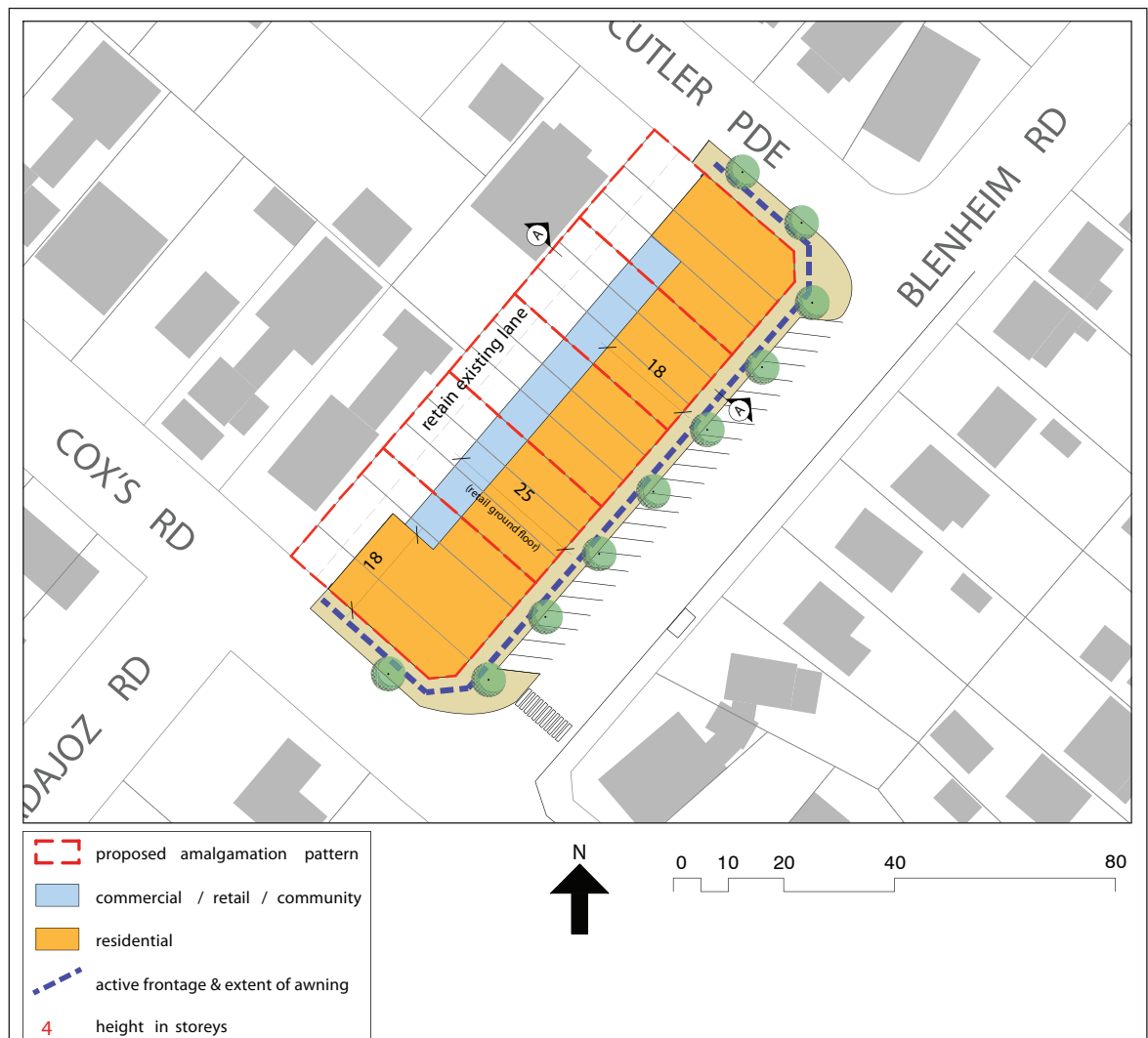
Figure 5.4.07 Blenheim Road Small Centre Building Depth Control / Active Street / Extent of Awning Control
