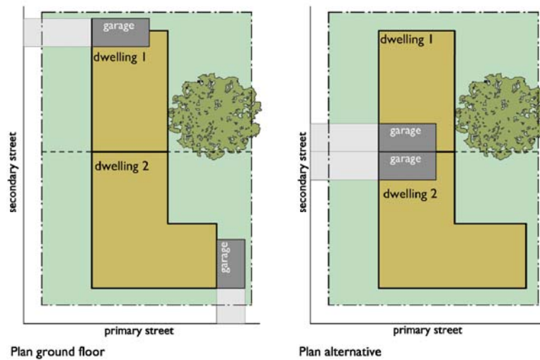
Figure 3.3.04 Alternative arrangements for a dual occupancy (attached) building on a corner allotment. Where dual occupancy (attached) dwellings have adjacent garages, the driveway does not need to narrow to a single driveway width.
