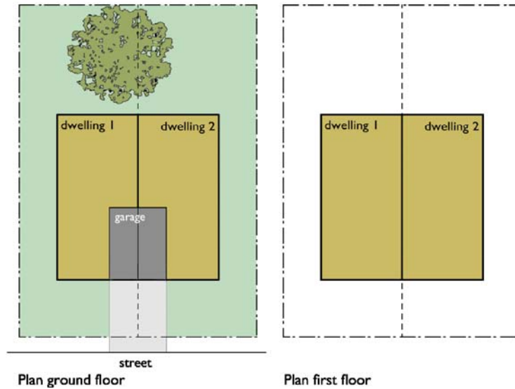
Figure 3.3.03 Illustrative plan of a dual occupancy (attached) with car parking at the front.
