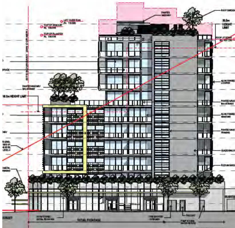
South elevation – after amendment – top level deleted.
