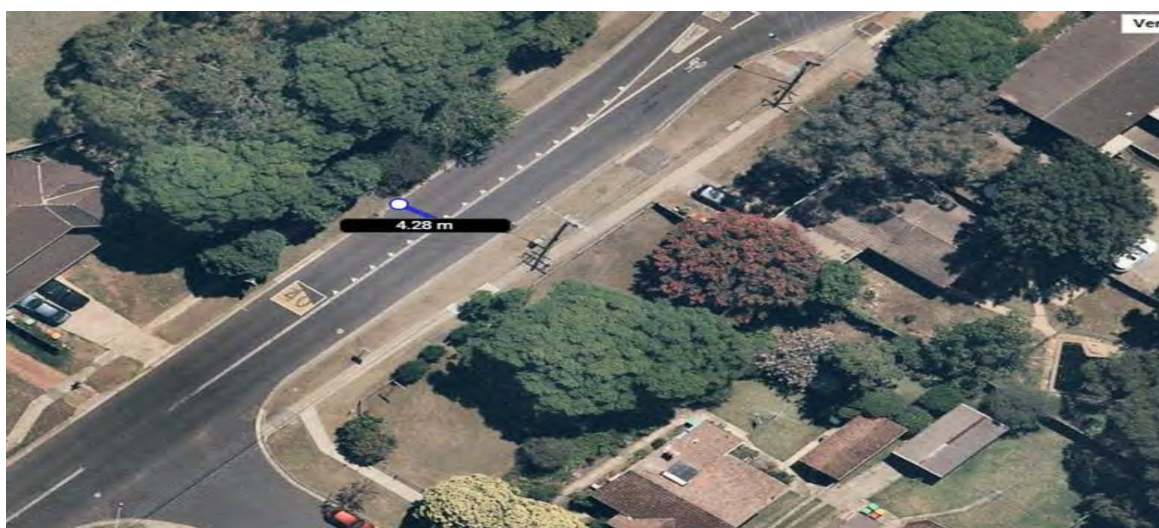
Figure 7: Proposed relocation of double barrier lines by 1m to permit legal parking on the eastern side of Herring Road
