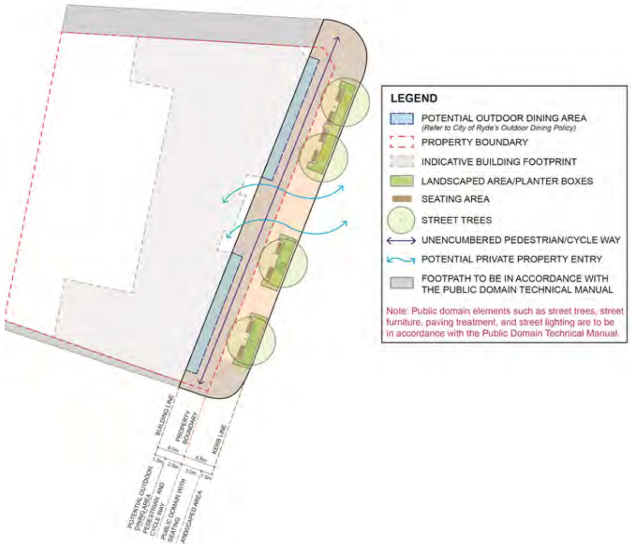
Figure 1: Indicative Urban Plaza Diagram (prepared by Council staff) for inclusion in the draft amendments to Part 4.3 of the DCP.
