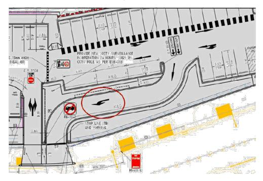
Figure 4: Combined Access Point - Showing Left Turn Only Egress Point
