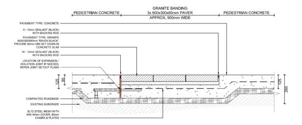
Figure 3.3.3 Detail: Granite banding in concrete footpath
