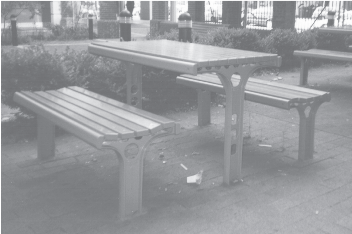
Figure 9.2.07 Leg of table prevents use by wheelchair user
