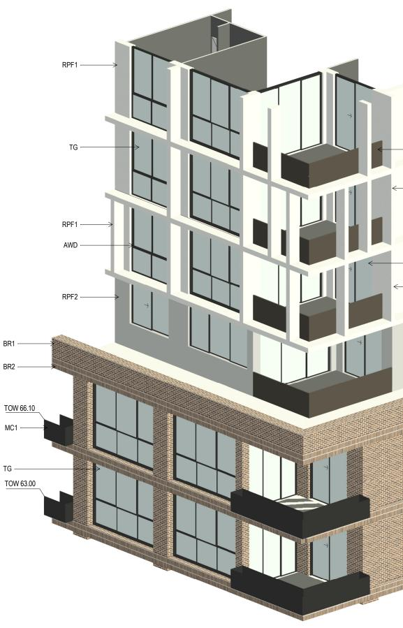
1 **BUILDING C - FACADE DETAIL ELEVATION**
