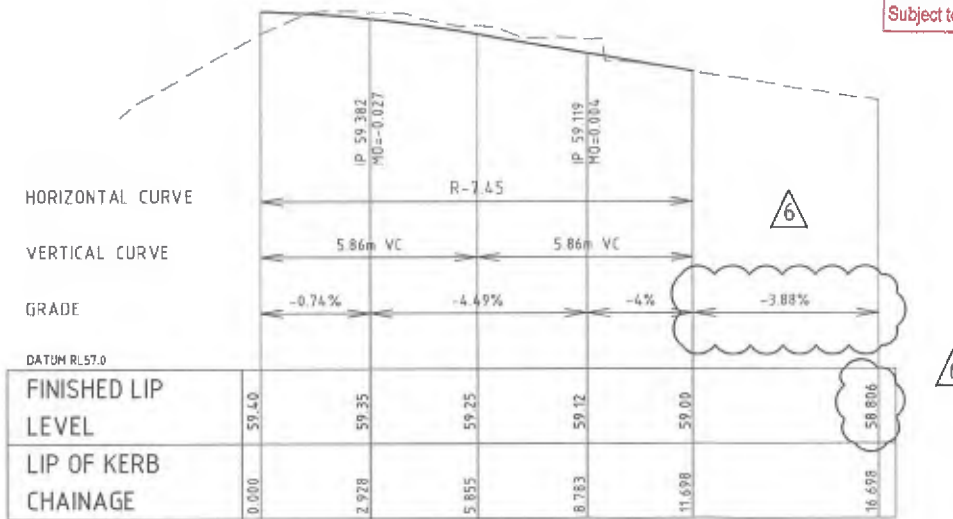
SCALE 1:100 HOR - 1:25 VER LONGITUDINAL SECTION ALONG KR002
