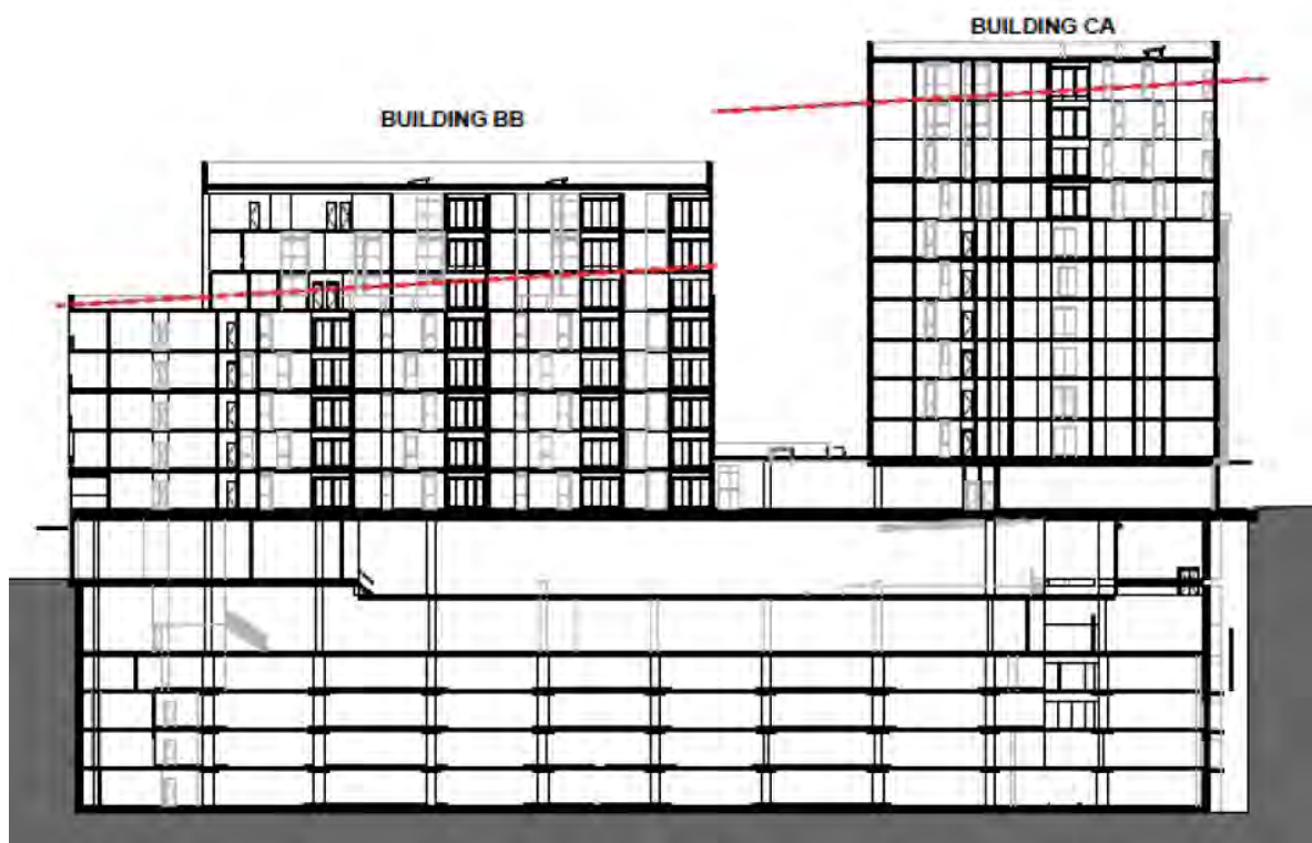
Figure 25. Section through Buildings BB and CA showing the height variation. The red line represents the applicable height control.
