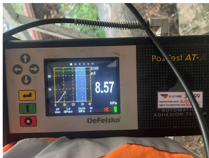
Figure 20- Adhesion pull-off test
