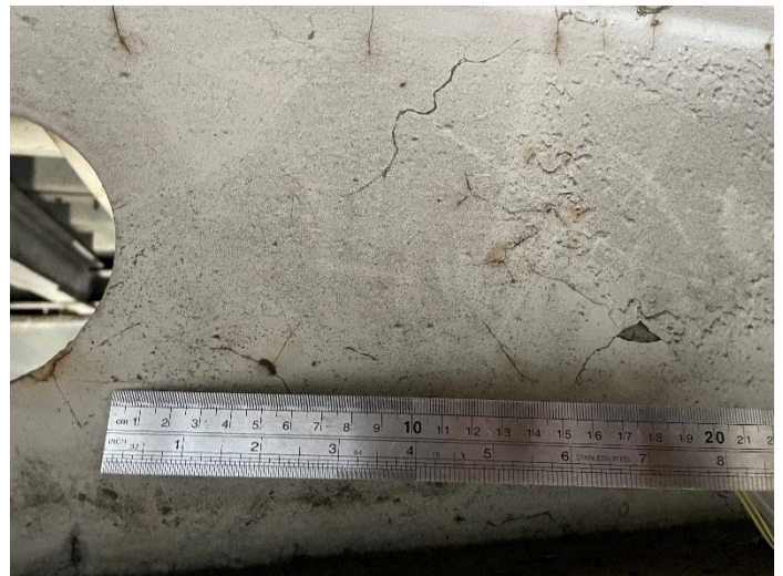
Figure 4- Flaked coating on transom
