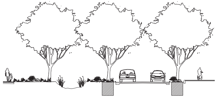
Creek corridor with naturalised, soft edge channel Bioretention System Road with 1.5% fall Bioretention System
