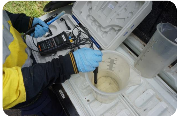
Figure 6 In-field water quality testing
