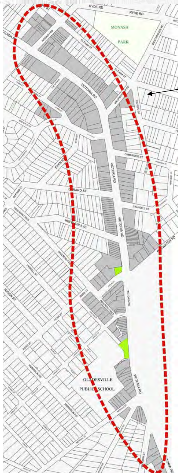
Figure 16. Extent of under-grounding of overhead services
