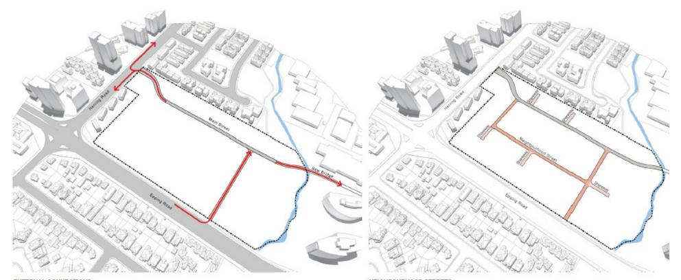
EXTERNAL CONNECTIONS A new bridge over Shrimptons Creek will provide vehicular and pedestrian connection to Lyonpark Road and the Employment Precinct to the east. A new road connection to Epping Road further links Ivanhoe to the broader street network. NEIGHBOURHOOD STREETS A regular grid of neighbourhood streets provides a clear network of circulation routes and access points.
