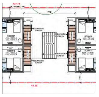
Figure 21 - 5.3m internal balcony and 7.7m building separation is proposed
