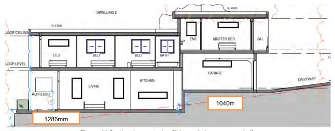
**Figure 11** Section demonstrating fill beneath the garage and alfresco.
