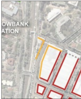
Figure 3 Figure 4.2.12 Setbacks diagram nominating a nil setback applicable to the site's E and W boundaries
