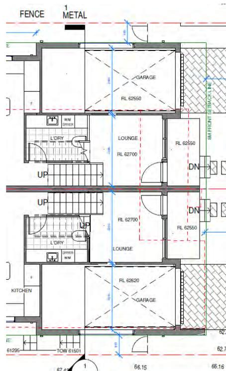
**Figure 13** The garages do not comply with the 1.5m setback control for 2 storey dwellings.
