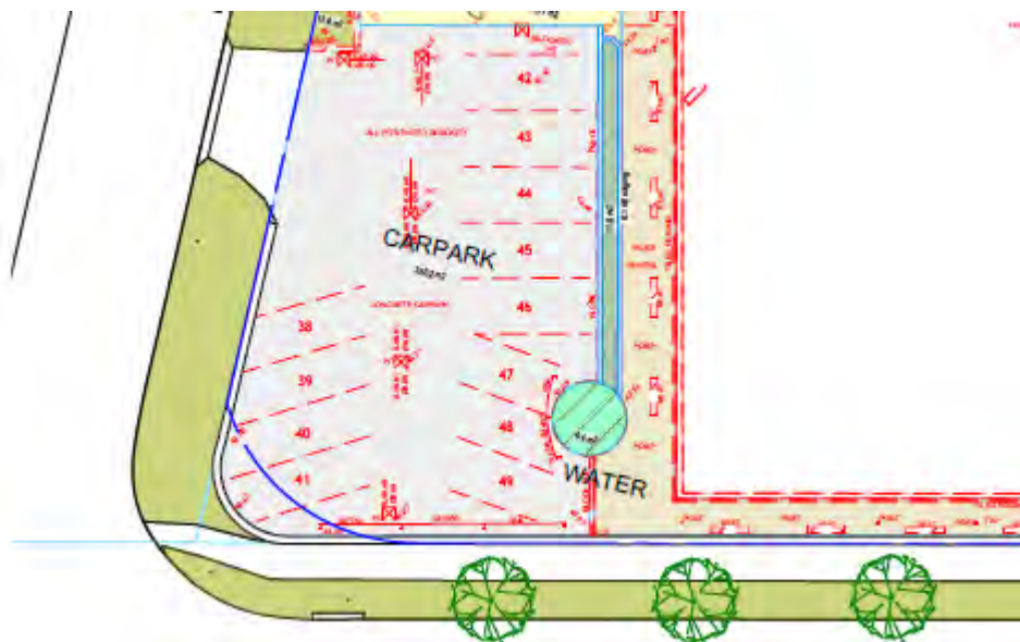
Figure 19 – The blue line represents the property boundary at the corner of the site near Swan Street and Ryde Road. The sandstone retaining wall encroaches into the public domain
