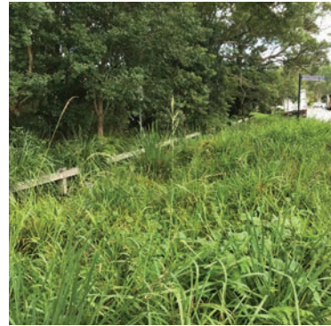
Planted strip of vegetation between access way or paved areas and native vegetation to provide stormwater filtration.
