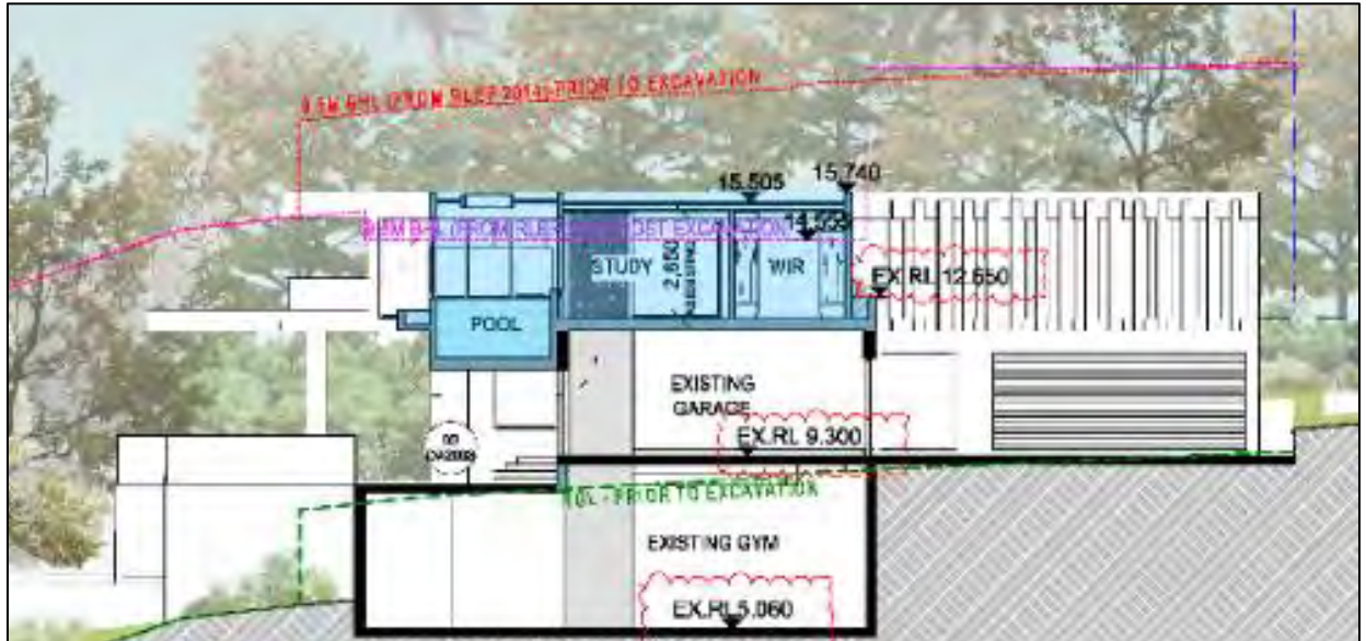
Figure 16: Building Height non-compliance shown in pink. The area above 1.180m shows the section of the dwelling which is non-compliant with height as a direct result of the topography with the previous excavation shown in green for the basement area.
