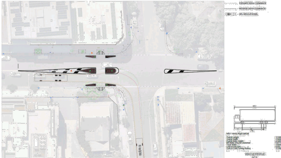
Figure 3: Swept path assessment for a 12.5m long HRV
