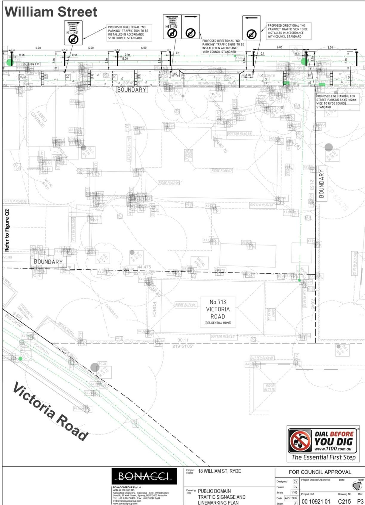
Figure P3: Signage and Line Marking Plan – Part 2
