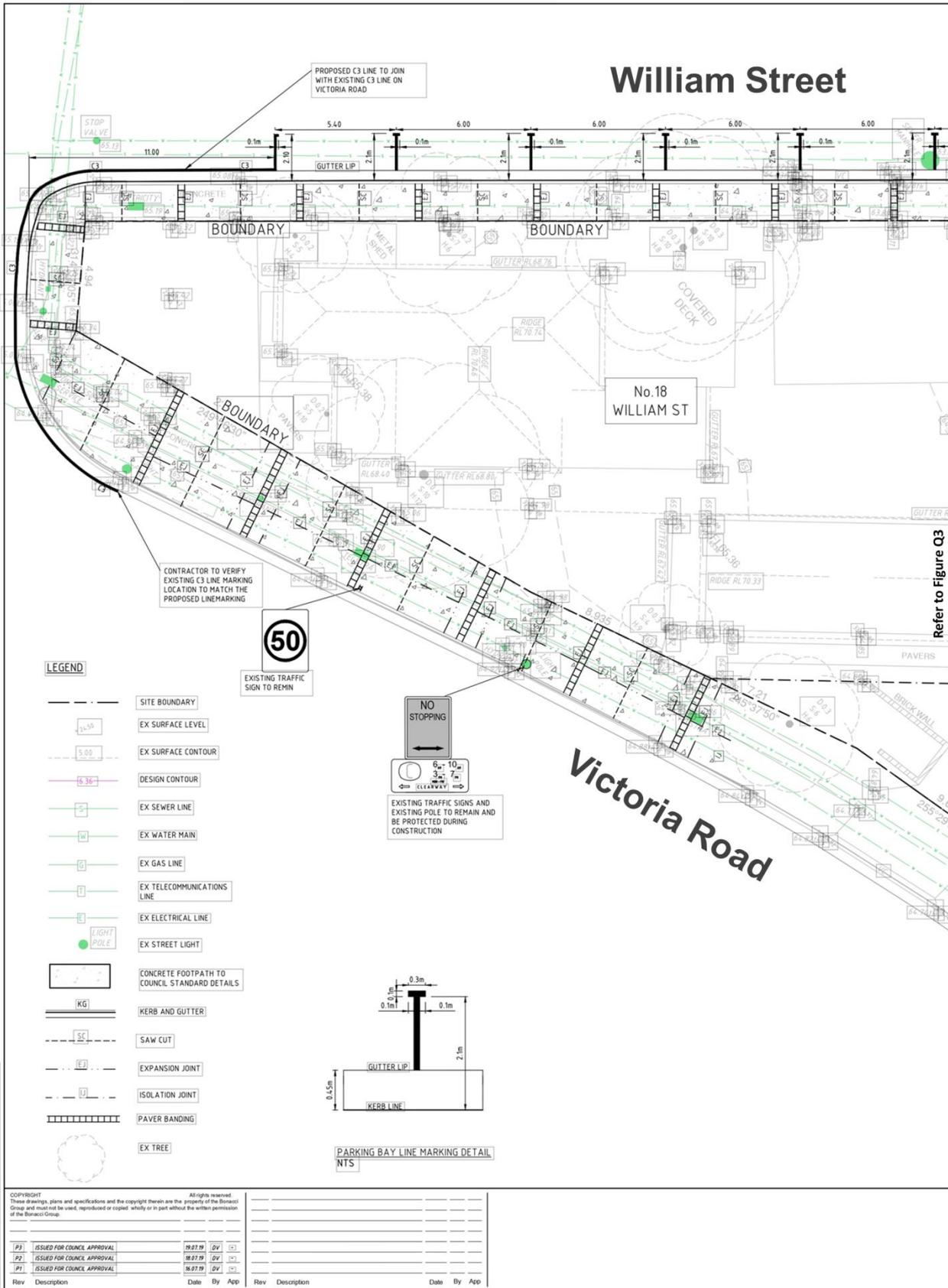
Figure P2: Signage and Line Marking Plan – Part 1
