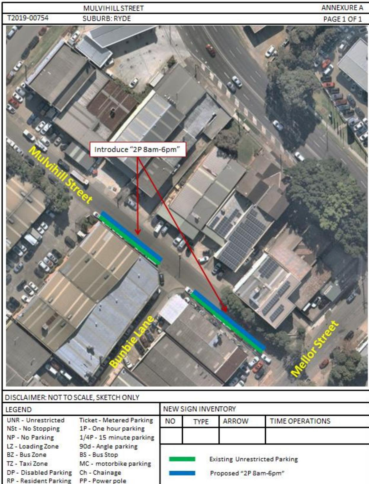
**Figure D2: Proposed 2P 8am-6pm Parking Restriction**
