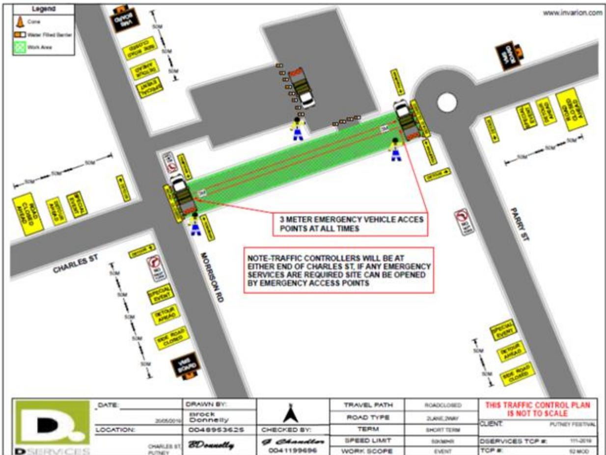
Figure Q1: Vehicle Management Plan
