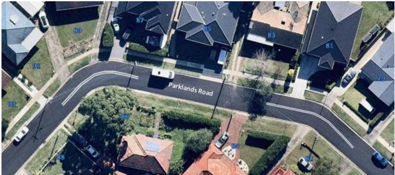
Figure 2: Proposed Location of Double Barrier Lines
