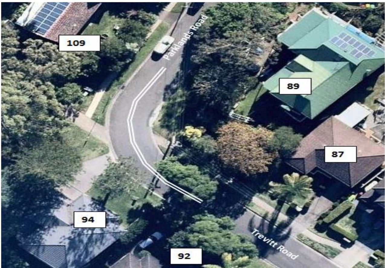
Figure 3: Proposed Location of Double Barrier Lines
